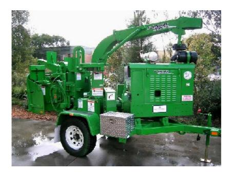
The **Model 90XP** is a compact, easy-to-tow 9-inch capacity disc-style chipper.
